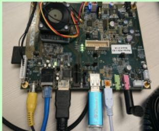
**BSP (Board Support Package )** = subset of SDK, designed for specific target hardware. **Embedded SoC vendor develops BSP for their reference platform.** Product producer modify BSP to fit with product hw
